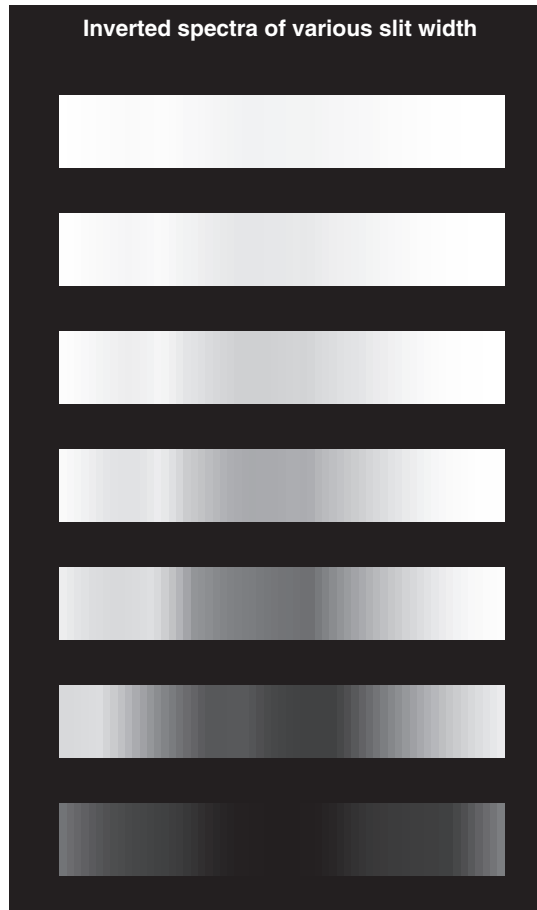
Figure 1.17 The inverted spectrum at various slit widths. (See colour Plate 8 in the centre of this book.)
